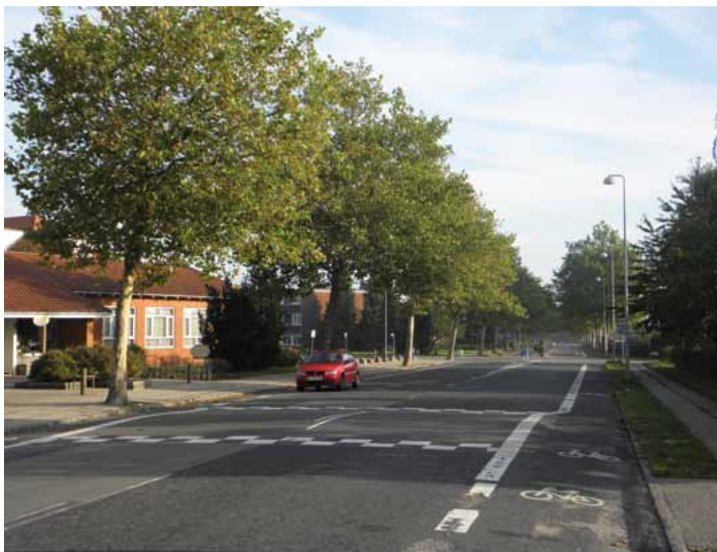
Cycle lanes combined with speed humps are reasonably safe and secure.
