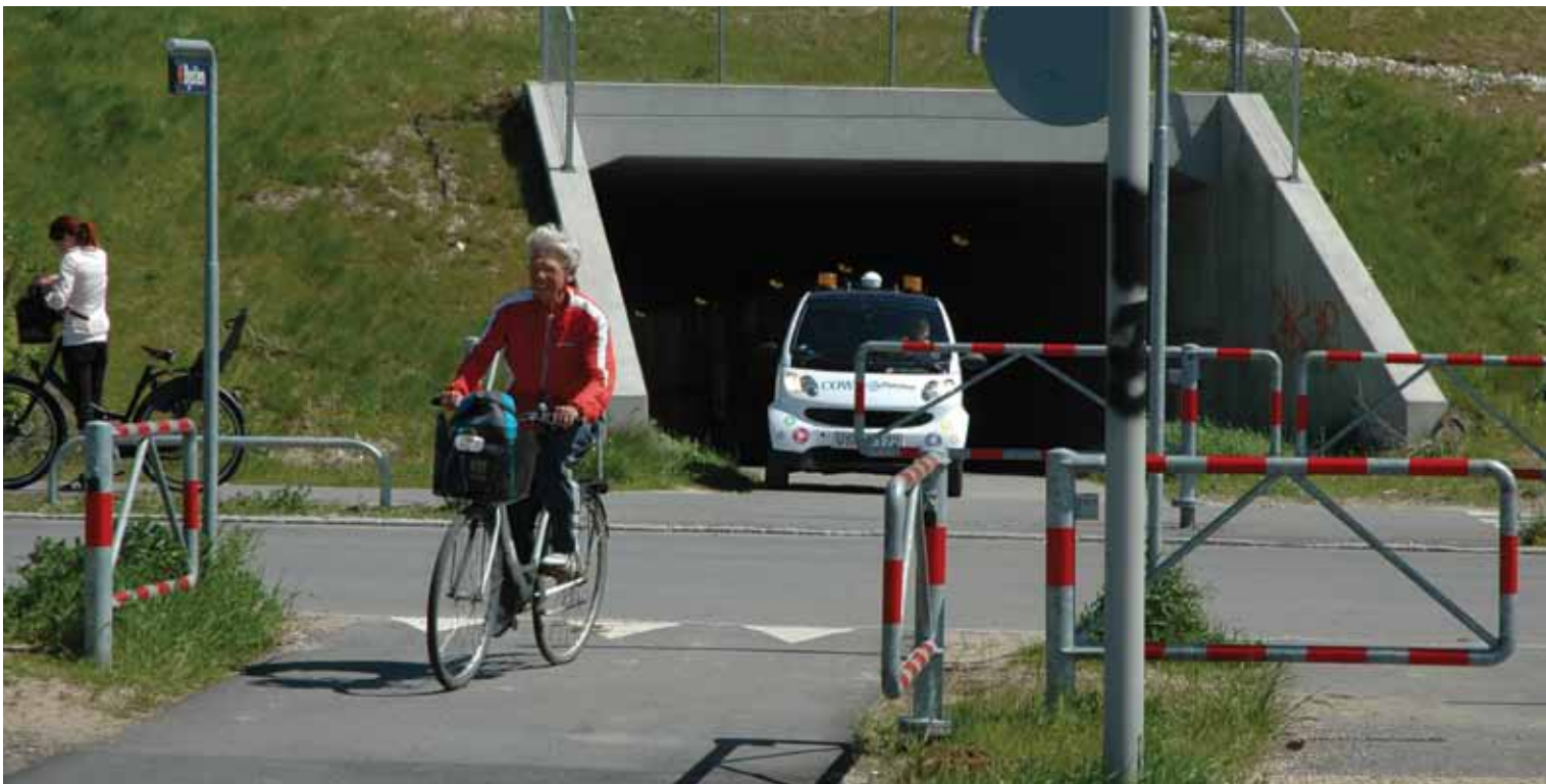
Road surface measuring vehicle equipped with laser devices. A sign on the back of the van explains why the van is on the cycle track.
