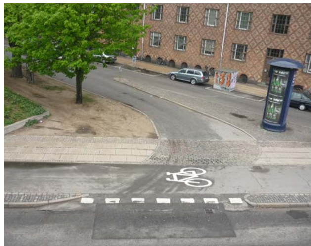
Continuous footways in Copenhagen – with footway materials continued through (left) and varied (right)
