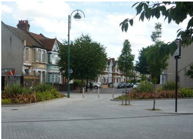
Modal filter with greening and folding bollards, Leytonstone
