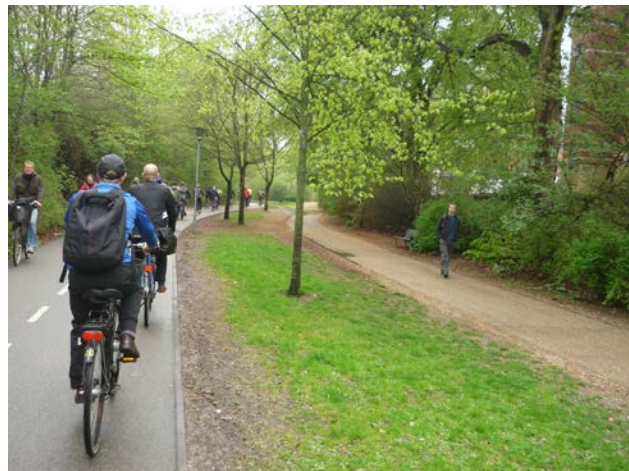
Separation by level difference in areas closed to motorised traffic – (left) Separated track and footpath in Copenhagen and (right) Steatham Street, Camden
