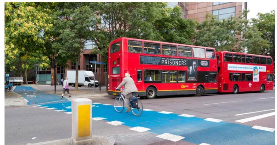
Signal-controlled cycle crossings, using elephant's footprint markings through the junction
