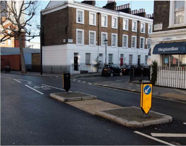
Pedestrian refuge island assists cycle right turn
