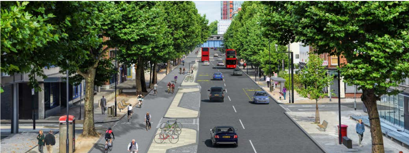
Visualisation of Cycle Superhighway scheme for Blackfriars Road, where side roads and active uses are predominantly on the east side and a two-way track is therefore proposed for the west side.
