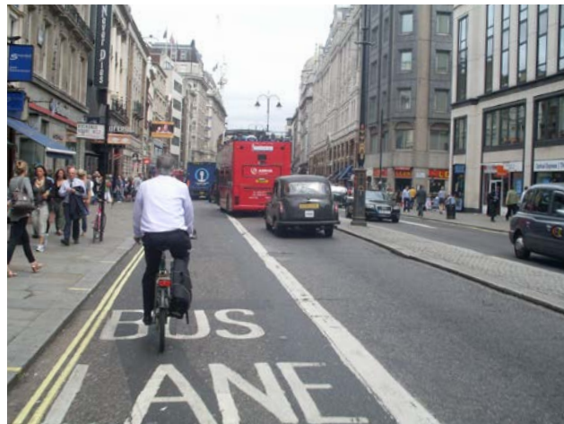
With-flow (left) and contraflow (right) bus lanes – note that ‘bus and cycle only’ marking is no longer prescribed
