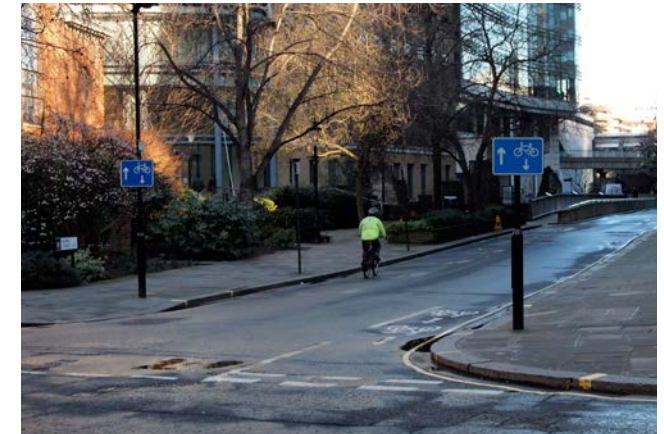
Contraflow cycling in City of London using the diagram 960.2 sign: advisory contraflow at Aldermanbury Street (left) and at Noble Street (right) using advisory lane markings only at the junction
