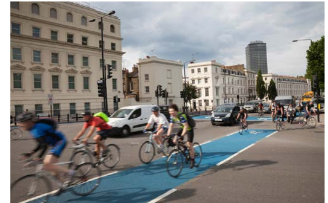
Lane markings and surface colour continued through junctions on Cycle Superhighways
