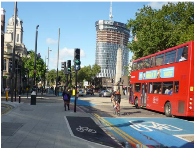
Dropped kerb providing cycle access to shared use footway and shared crossing
