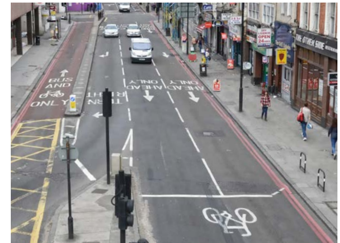
With-flow (left) and contraflow (right) bus lanes – note that ‘bus and cycle only’ marking is no longer prescribed
