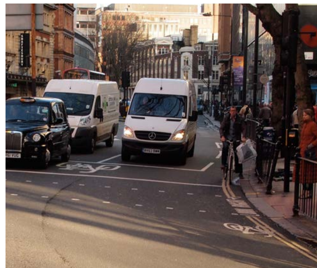
Well-placed cycle symbols through a junction to show a recommended route for ahead cyclists (top). Poorly placed cycle symbol on a bend (bottom)
