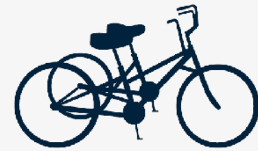
Side-by-side tandem L 1800-1950mm / W <1070mm
