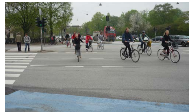
Two-stage left-turn marking at junction in Stockholm (top); and cyclists in different streams in Copenhagen (bottom) – left turners are heading to the waiting area to the right
