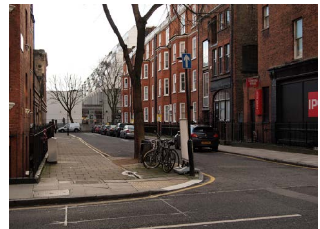
Footway build-out incorporating cycle parking
