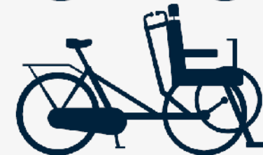
Tricycle, including wheelchair-friendly model L 1400-2100mm / W <850mm
