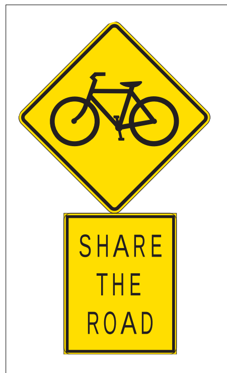
Figure 7- 6: Share the Road sign MN MUTCD Sign W11-1 and W16-1
