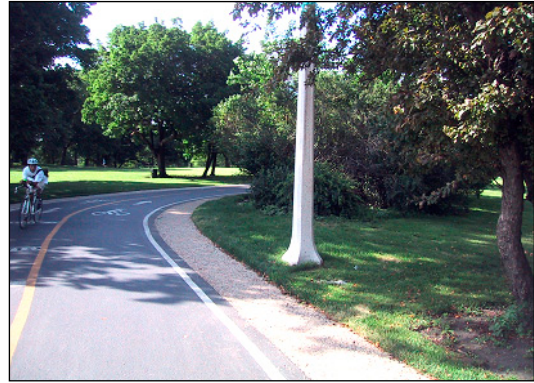
Figure 5-7: Example of unacceptable sight distance on a curve
