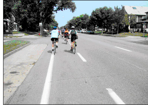
Figure 4-15: Left Side Bike Lane on a One-Way Street
