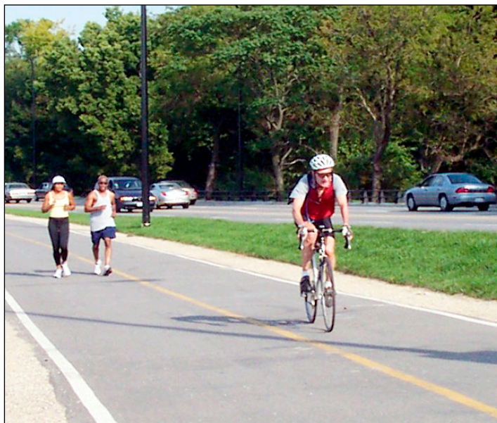
Figure 5-5: This shared-use path is separated by at least 3 m (10 ft) from the roadway
