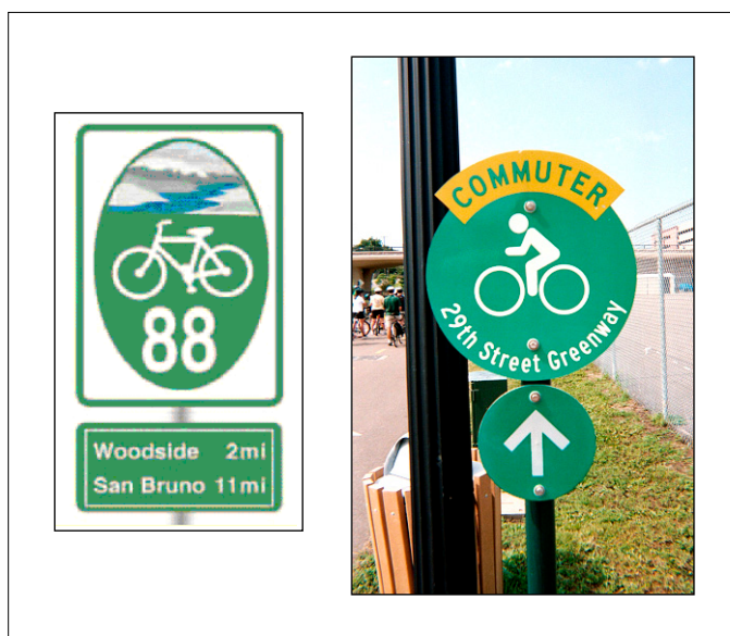
Figure 7-7: Examples Special Bikeway Signage
