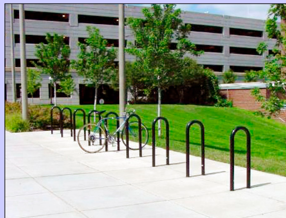
Figure 8-9: Inverted-U Bicycle Rack
