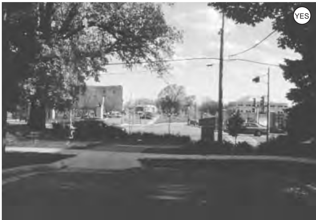
Figure 2-65: A street closure keeps major street traffic from diverting onto this residential street. The short path (foreground, left) connects the neighborhood with a signalized crossing and the school beyond.
