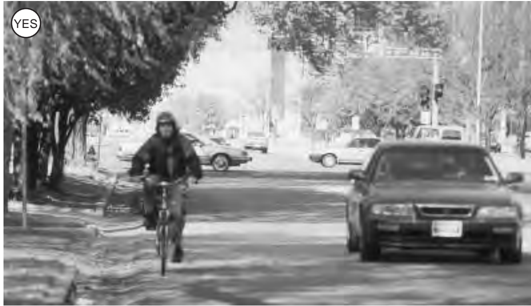
Figure 2-4: Collector streets like this one typically carry lower traffic volumes and have lower speeds than arterial streets. As a result, many bicyclists feel more comfortable using them.
