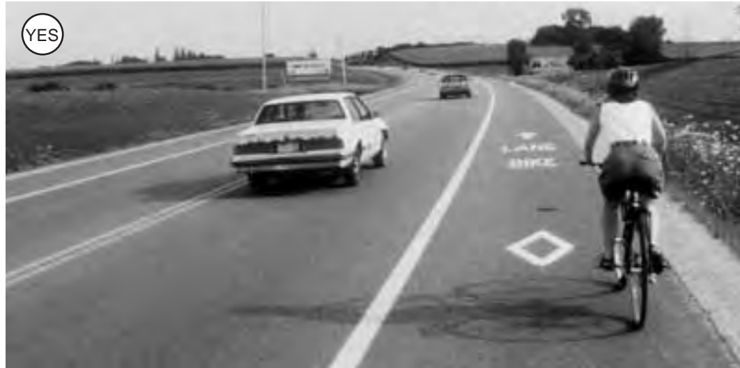
Figure 2-32: Adequate paved shoulders on rural roads provide clearance between bicyclists and passing motorists. In this particular instance, the shoulder is marked as a bike lane, since it links a state park entrance and a state trail.
