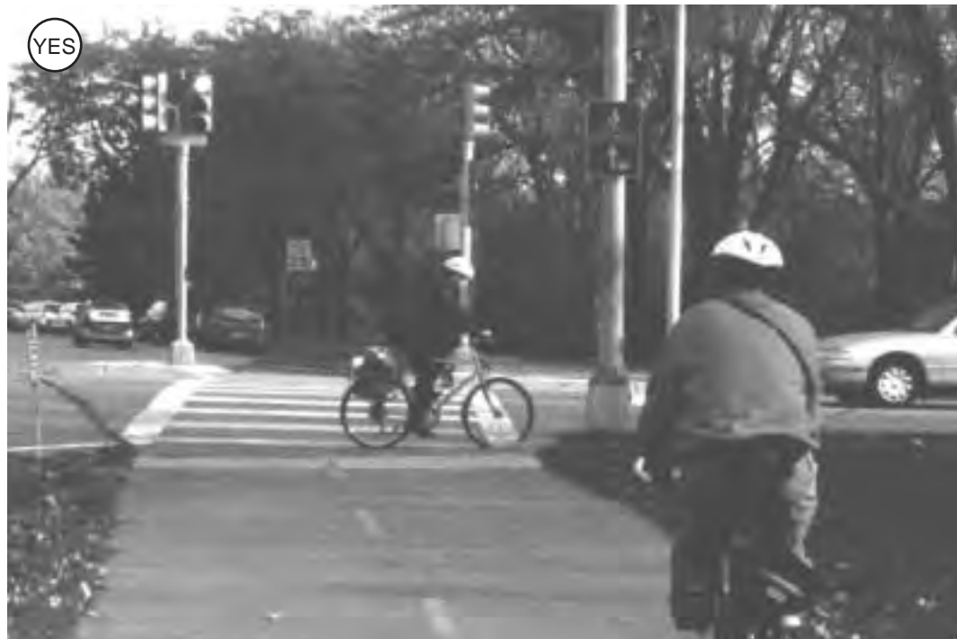
Figure 4-106: An urban crossing that takes advantage of an adjacent signalized intersection. A bicycle signal loop detects bikes to change the signal. Note high-visibility crosswalk marking.
