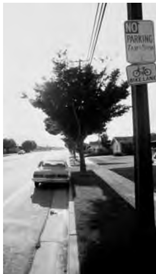
Fig. 3-7: Part-time bicycle lanes are not recommended except in very special situations. And they require vigilant enforcement.
