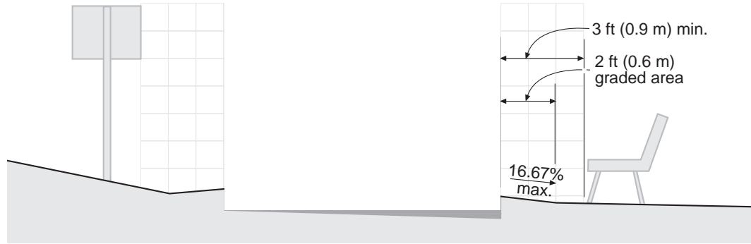
Figure 4-11: Maintaining adequate shoulders and proper clearances between the path and obstacles preserves the path's effective width.
