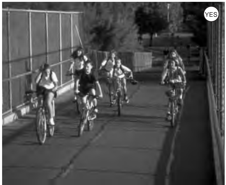
Figure 4-10: One-way paths are often used in two directions unless paired with another nearby one-way path.
