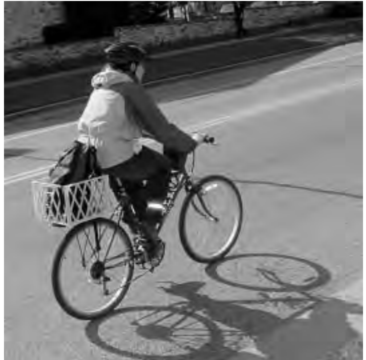
Figure 1-5: Typical speeds range from 7 to 15mph for average bicyclists.
