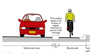
(c) Adjacent bicycle path (part of road surface) with separating kerb. Width of separating kerb: 0.4m no parking; 1.0m with parking or where pedestrian activity is high. Bicycle path can be one-way or two-way.
