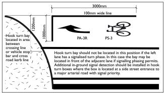
box at a large cross intersection. This box should be no longer than 3.0m and 1.0m wide. It should be located in a 2.5m wide area immediately in front of the pedestrian crossing area and not protrude into the adjacent crossroad kerbside travel lane. Hook turn boxes should always be placed so that they do conflict with left turn signal phasing. Additional signal detection should be considered where hook turn boxes are placed at side street entrances to major arterial roads.
