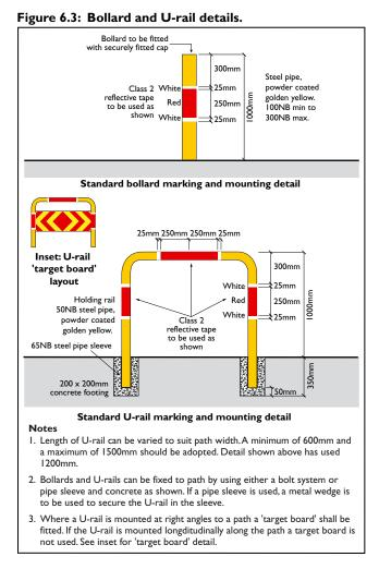
clearances for riders and pedestrians. Bollards should be finished in a light bright colour with reflective tape to make them highly visible to road and path users in low light conditions (see Figure 6.3).
