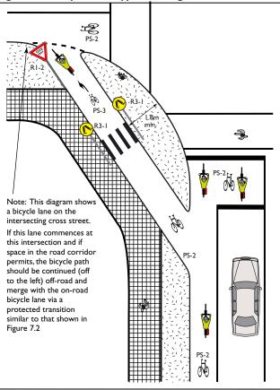
7.20 shows a left-turn bypass for riders at a signalised intersection. The concept behind this treatment is similar to Figure 5-21 in Austroads – Part 14.
