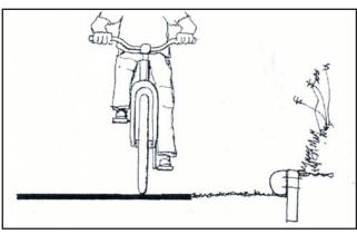
Figure 8.5: Clearances should be maintained on path edges to provide a safe and level run-off area.
