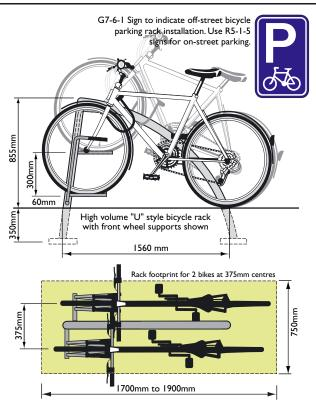
Figure 11.2: High volume bicycle parking installation.
