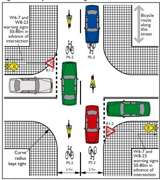
Figure 7.11: Bicycle route through mixed traffic roundabout.
