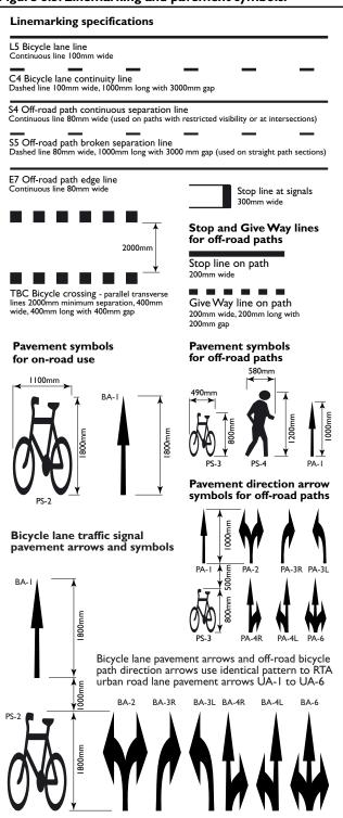
Austroads Guide to Traffic Engineering Practice, Part 14 – Bicycles (Section 9.6, Pavement Markings), provides linemarking guidance for both on-road and off-road facilities. The information provided below is additional to this guidance.
