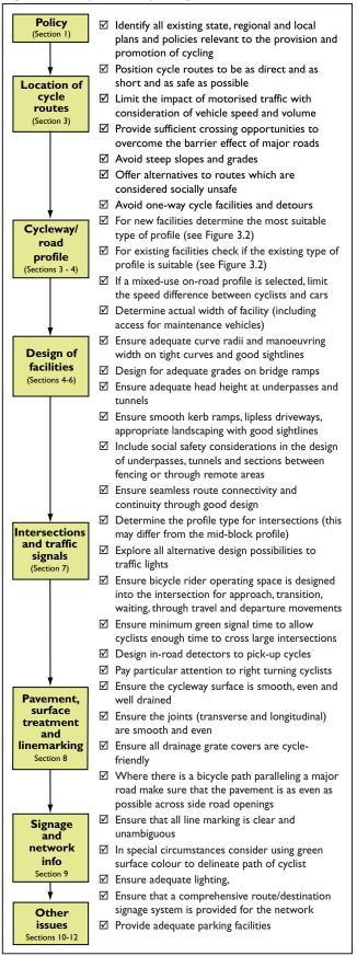
This section explains the design principles and the philosophy which underpin this manual. Figure 3.1 provides a simple checklist which can be used to follow the decision process through the various sections of this document.
