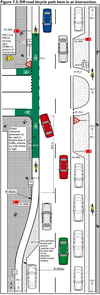
**cle path bent-in at intersection.** the design process when p for unsignalised intersectio
