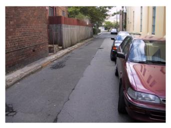
lane widths wider than 2.6m should be avoided as excess width increases the possibility of risky overtaking behaviour. Any excess street width should be allocated to the parking lane rather than the travel lanes. A 2.6m lane on a two-way street will allow for emergency vehicle access.
