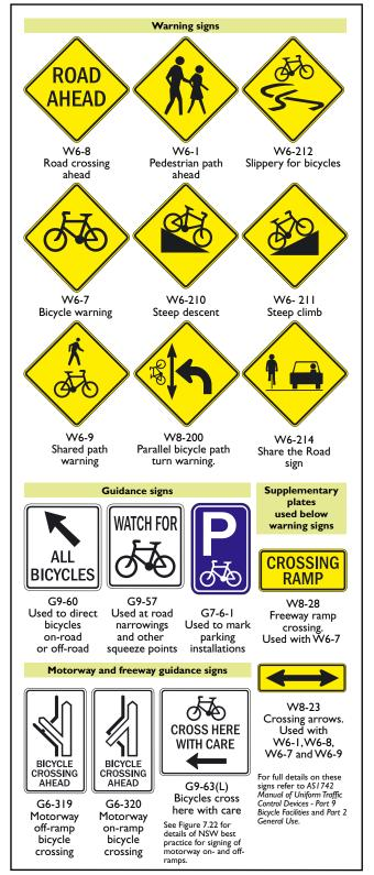
Figure 9.2 shows the most commonly used warning signs (and supplementary plates) for both bicycle network and general road network use.
