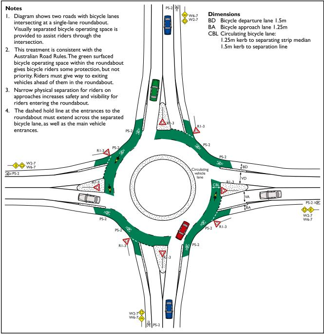
bicycle route passing through it. The route treatment in this example uses bicycle shoulder lanes. There are numerous examples of this type of roundabout in operation. It is suitable where vehicle speeds are 50 km/h or less.
