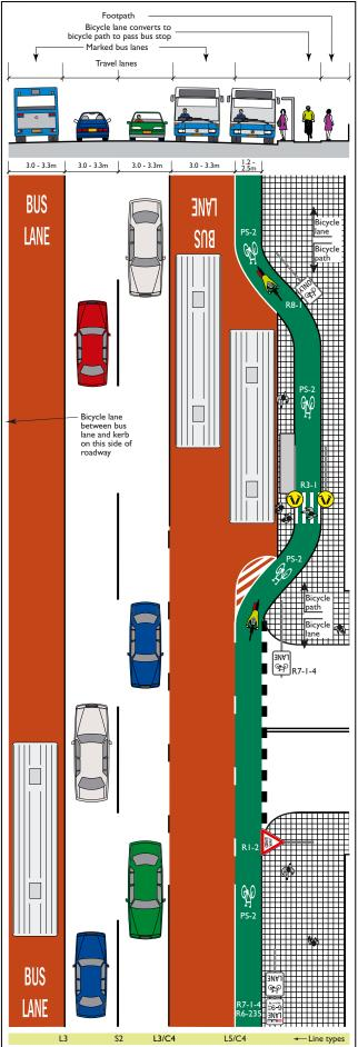
must pull into the kerb to pick up passengers. This means that bicycle riders must deviate into the bus lane to pass a stationary bus.
