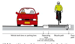
(d) Adjacent bicycle path (narrowed road surface) with separating verge of adequate width to allow for vehicle travel lane or adjacent car parking. Bicycle path can be one-way or two-way. New channels laid under bicycle path to deliver road run-off to existing drainage pits.
