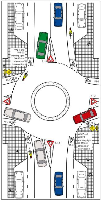
Figure 7.8: Bicycle route at small single lane roundabout.
