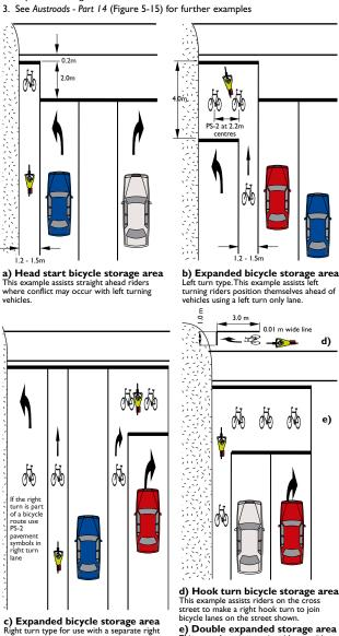
Right turn type for use with a separate right turn phase. Right turn box may be reduced to a head start area if lane guidance markings are provided through intersection.
