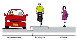
(b) Adjacent bicycle path with no separating verge. Not recommended where adjacent car parking is present or for a two-way bicycle path.
