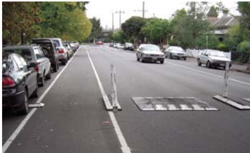
Speed cushions with cycle lane bypass, Melbourne, Australia. (Photo: Tim Hughes)
