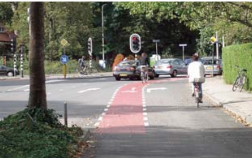
Coherence — Separate cycle path becomes cycle lane to continue through signals, Delft, The Netherlands. (Photo: Tim Hughes)
