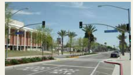
Although not raised, this mid-block crossing in Fullerton outside the City Hall features curb build-outs and different surface material
