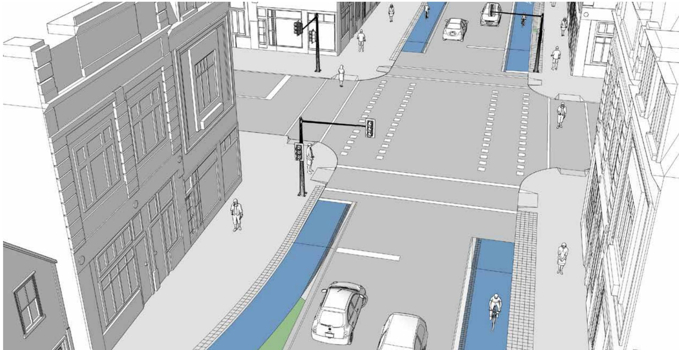
Unprotected intersections are intersections where cyclists are more exposed to traffic due to a lack of corner safety islands. Cyclists mix with vehicle traffic on the intersection and with pedestrian traffic where they cross the crosswalk.
