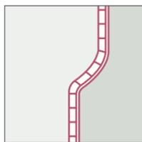
Footpaths make up the majority of the network of pedestrian facilities. The clear through route on any footpath should never be less than 1.8 m wide. Footpaths should have hard, even paving and crossfall of 2% (not more than 3%). Footpaths should include a buffer between the clear path and traffic; presenting a good place for street furniture, utilities and service covers and tree pits. Space for commercial activity should be provided in commercial, retail and mixed-use areas.
