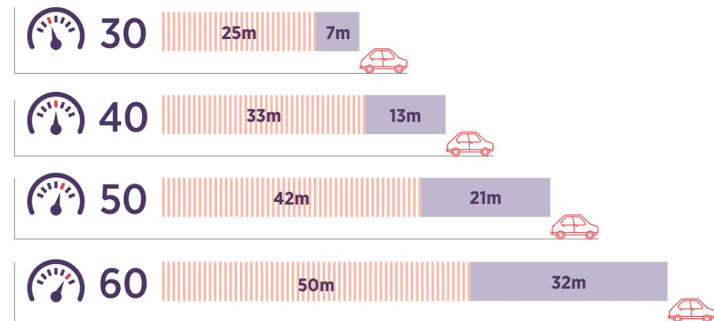
Perception and Reaction distance - constant speed (3s) | Braking distance (d=0.49 at 30 k, 0.48 at 40 k, 0.47 at 50 k, 0.45 at 60 k)
