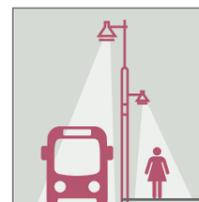
Pedestrian connections should be sufficiently lit to ensure safety, deter crime and create inviting spaces. Lighting should be scaled to the pedestrian, with lighting fixtures placed on all streets at appropriate intervals. Separate fittings will often be required for pedestrians and vehicle traffic. Commercial areas will be lit more intensely, whereas lighting in residential areas should be subtler. Lighting fixtures should not obstruct walking paths.
