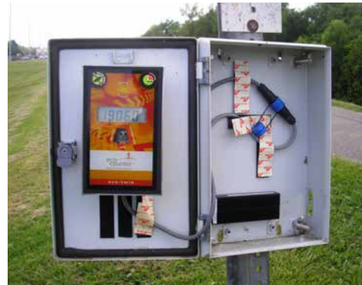
Figure 8: Detail of Eco-Counter Infrared Sensing Device
