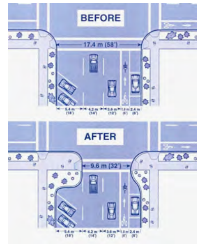
Curb Extensions - Before and After
