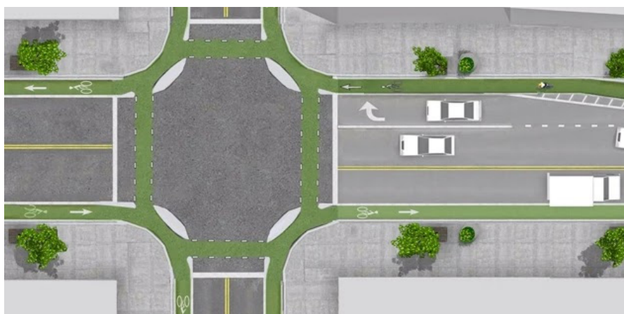
Figure 1: Dutch junction design features continuous designated bike lanes protected by curb islands. Source: Biotic Design Studio
