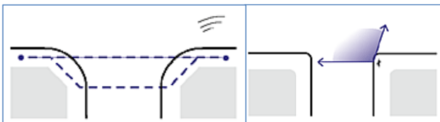
Figure 4-33: Large Radii Increases Desire Lines and Sight Distances
