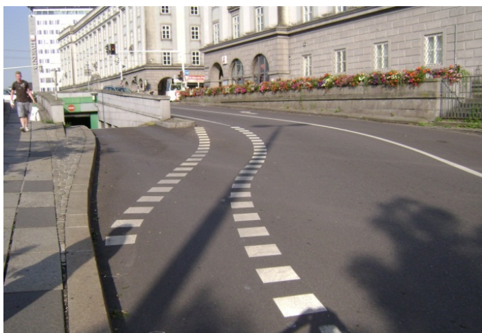
Figure 5-1: RTM 9 Lines Delineating Bicycle Lane
