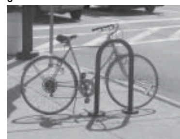
Select bicycle parking devices according to the need of the users and level of security required: 1) lockers for long-term secure storage, 2) racks that secure the frame and wheels for mid-term storage and 3) leaning rails for short-term low-security storage.
