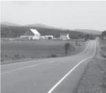
Paved shoulders can significantly improve operating conditions for motorists, bicyclists and pedestrians, especially in rural areas.
