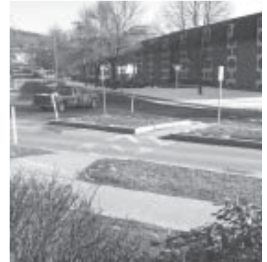
Position pedestrian crosswalks to bisect splitter islands.
