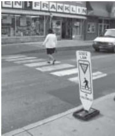
In street pedestrian crossing signs help communicate pedestrian right-of-way laws and alert drivers of specific crosswalk locations.
