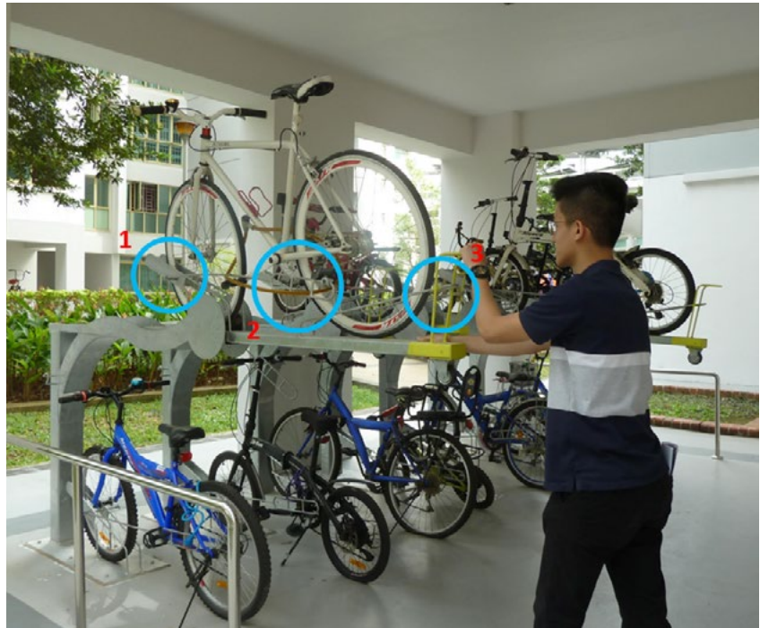
ABOVE: Bike racks should provide 3 points for secured bike parking
