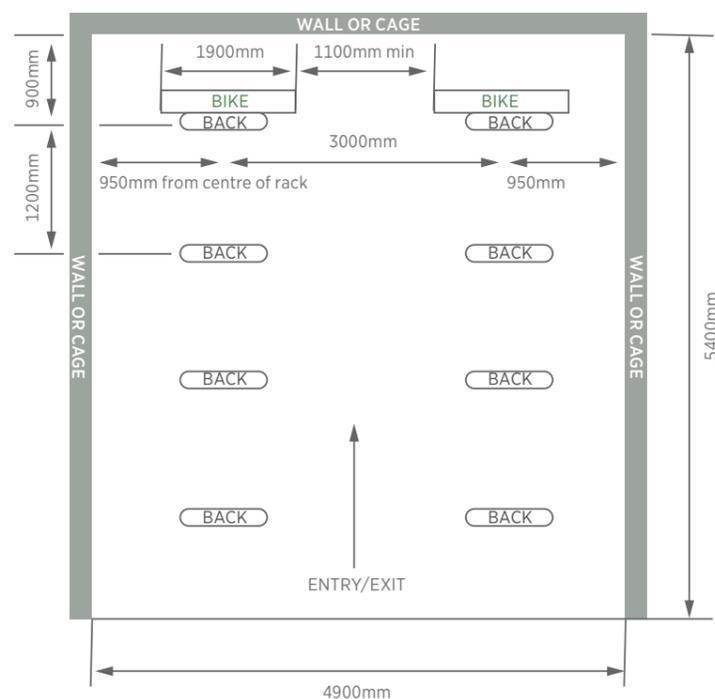
**Figure A.7** Long-term bicycle parking (for double sided stands, Sheffield only) layout for 16 cycles
