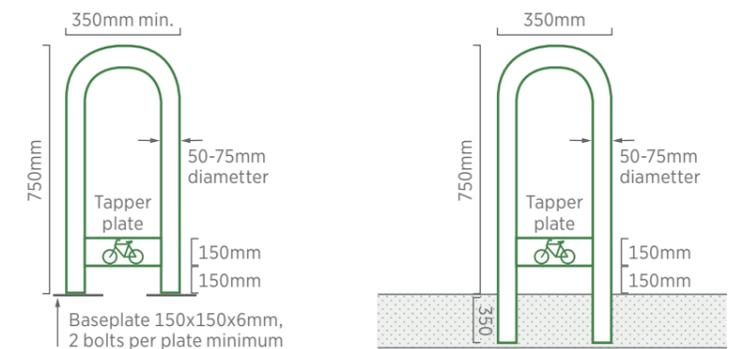
**Figure A.10** Harrogate bicycle stand dimensions. Left: surface mounted. Right: in ground
