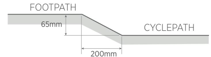
Kerbs not more than 70 mm high may be used at the edges of a cycleway next to a separator or buffer strip. These provide clearance for pedals.
