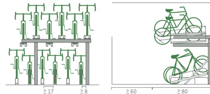
Figure A.11 Double-decker lift-assist bicycle racks
