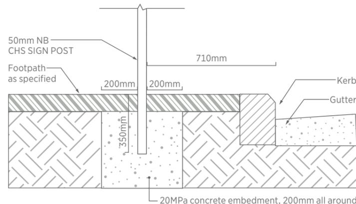
**Figure A.9** Required direct concrete embedment for a bicycle stand
