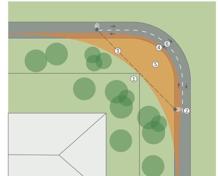
Figure 15 Lateral clearances on horizontal curves
