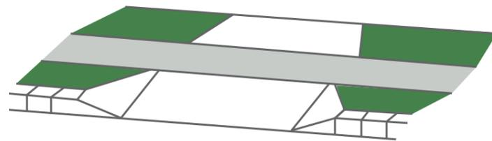
Figure 11 Surface treatment at vehicle crossing
