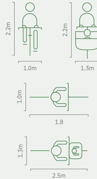
Most bicycles are about 1.7 to 1.8 m in length, and about 70 cm wide, with the height of the cyclist generally varying from 1.8 to 2.2 m. Larger bikes such as cargo bikes tend to be wider (up to 1 m) and longer, varying from 2 to 2.5 m. This has implications in all infrastructure where a person on a bicycle is present, from refuges and pram ramps to shared paths and separated cycle paths.
