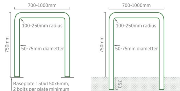
**Figure A.8** Sheffield bicycle stand dimensions. Left: surface mounted. Right: in ground
