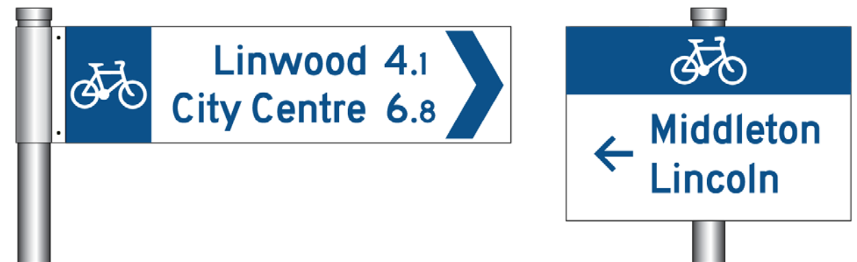
Figure 3.12: Typical size and location of the bicycle symbol shown in white on a blue background for primary route signage
