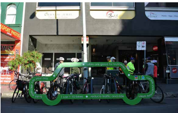
Figure 4.6 Clever bike rack designed to accommodate up to 12 bicycles within a single on-street car parking space, allowing footpaths to remain unobstructed
