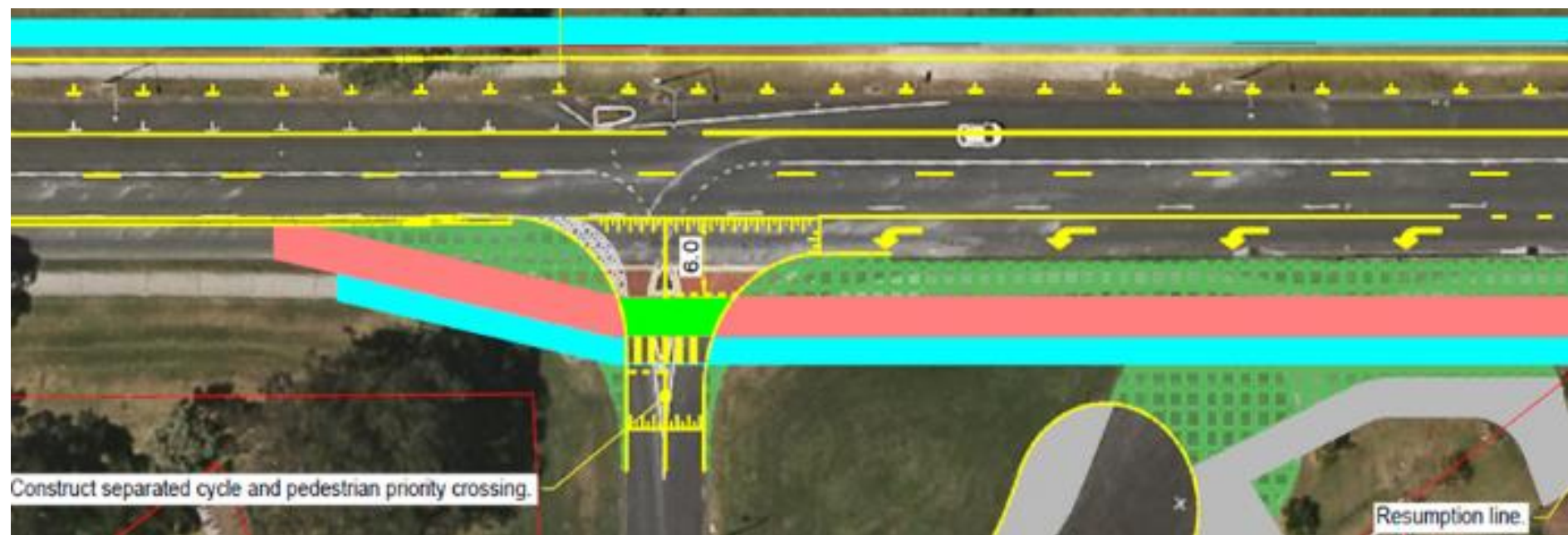
Figure 4.3.1(C) – Concept drawing of two-way cycle track with 6 m storage for exiting vehicles and 3 m buffer for vehicles entering from the added left-turn lane (LTS2)
