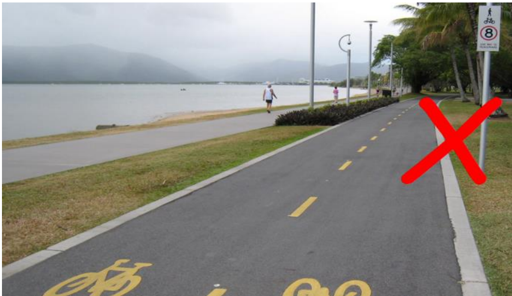
Figure 1.2(a) – Inappropriate speed limit signage application
