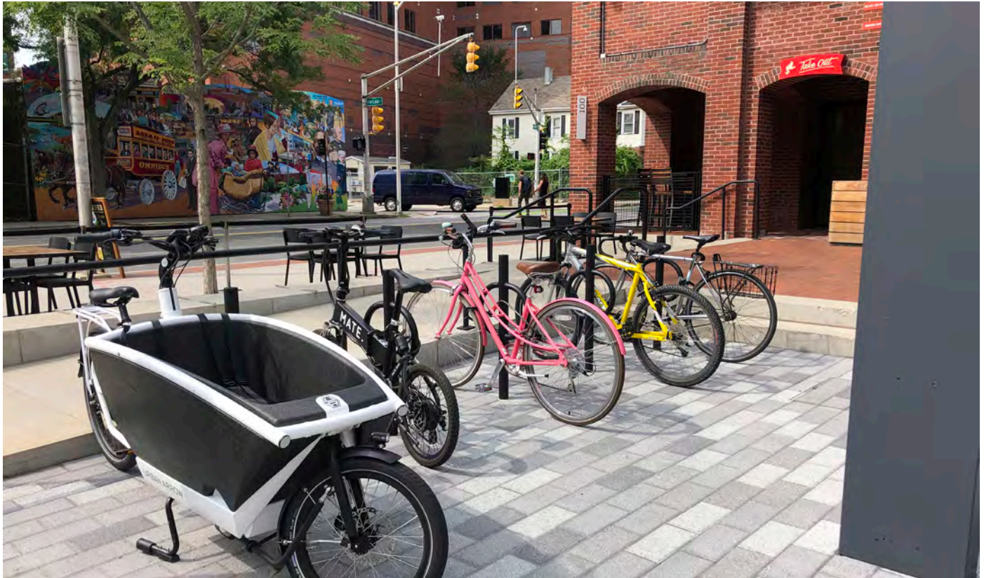
Figure 7.2: Bike rack designs need to accommodate the diversity of bike shapes and sizes, including cargo bikes and adaptive bikes.
