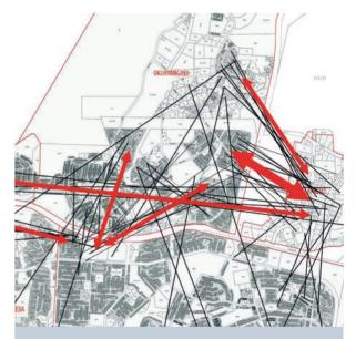
Fig. 13: Drafted Desire Lines for pedestrians of a quarter in northern Windhoek. Source: GIZ Transport Namibia, EBR 2016.
