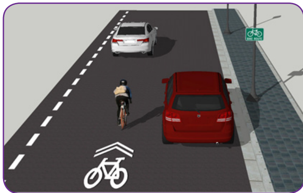
Figure 3-6 Class III Bicycle Facility
