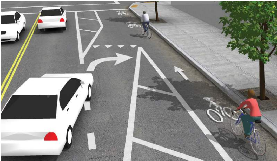
Figure 29 | Lateral shift design makes turning drivers aware that they must yield to cyclists going straight
