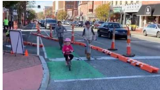
Figure 20 | Parked cars provide a buffer and help protect cyclists in the bike lane
