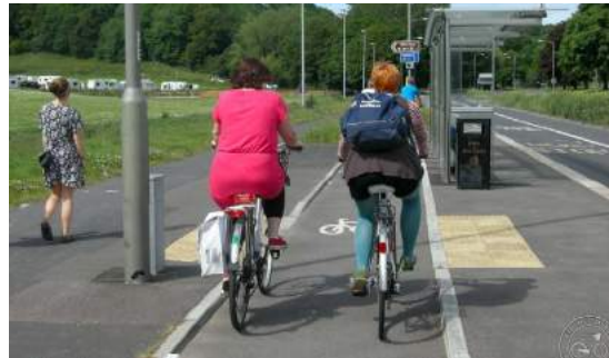
Figure 33 | Copenhagen-style bus stop in London, where bike lane is elevated and markings indicate that cyclists must yield to passengers
