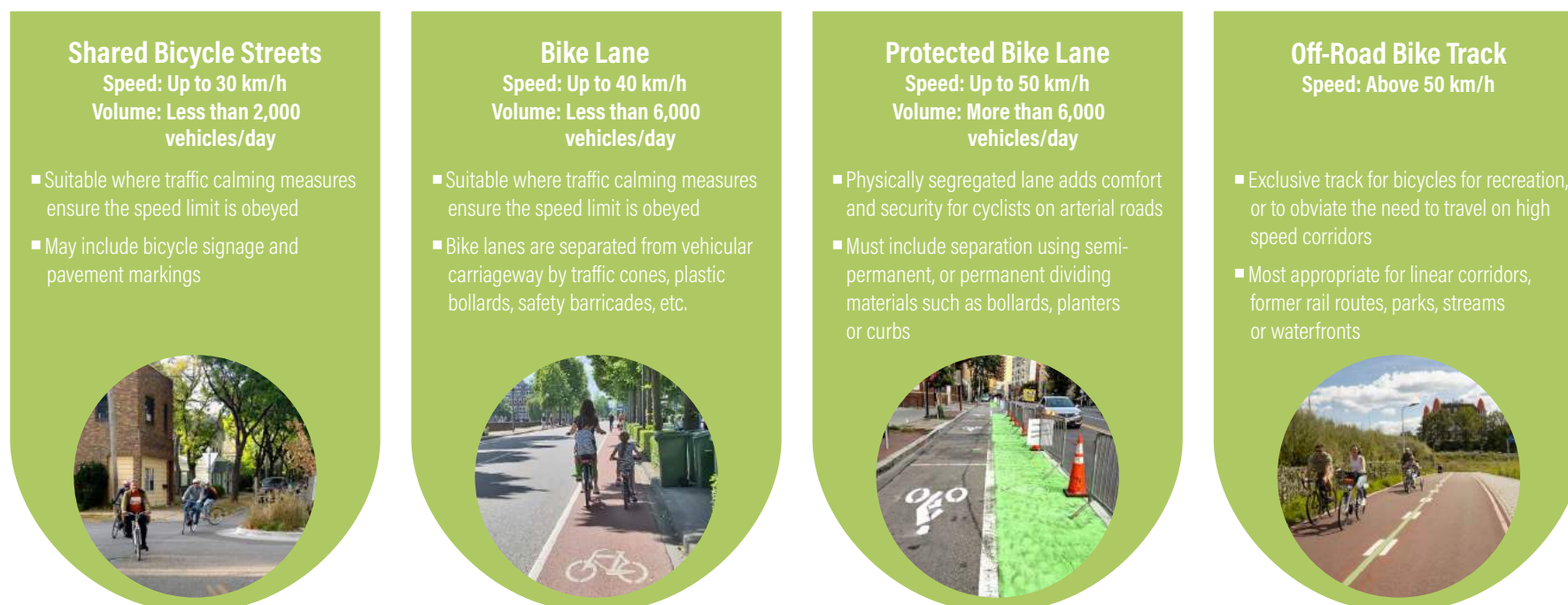
Figure 13 | Selecting appropriate bike infrastructure according to vehicle speeds
