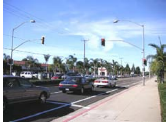
13S) This mid-block crossing utilizes standard traffic signals, a stop bar, ladder style crosswalks, median refuge and a pedestrian controlled actuator. Photo credit: Mike Singleton
