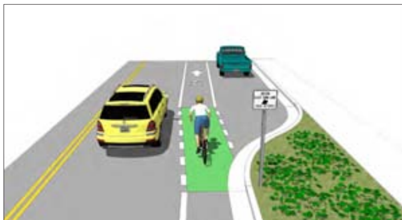
Example of a colored bicycle lane at high conflict areas with motor vehicles. Graphic credit: KTU+A
