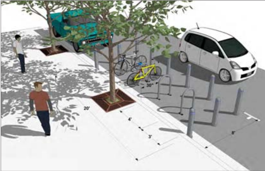
Dimensions for installation of a bike corral. Bike corrals convert one car parking space into 8-10 bike parking spaces. Graphic credit: KTU+A
