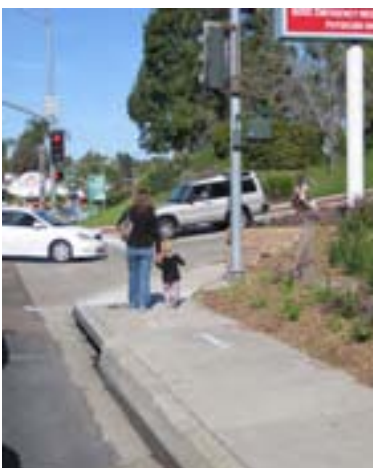
15S) Sidewalks placed against the curb, against a high speed and high volume street are not comfortable to walk on because of a fear (perceived or real) of being hit by a passing vehicle. Photo credit: Catrine Machi
