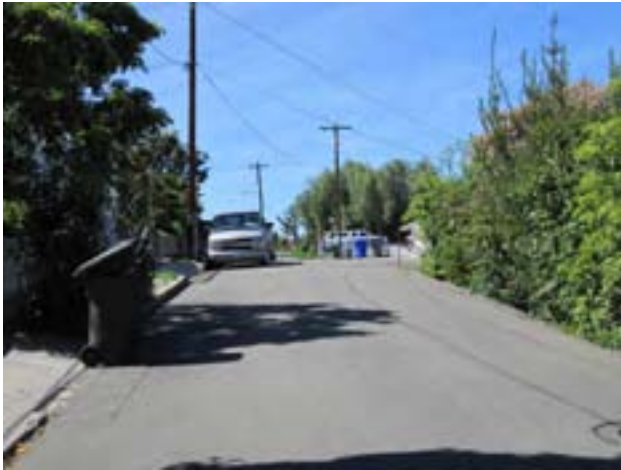
2C) In areas currently without sidewalks, where the street volume and speed is very low and the character is rural, sidewalks may not be needed. Photo credit: Joe Punsalan
