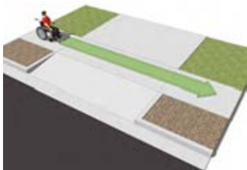
5A) A walkway separated from the curb with a parkway strip is the preferred solution. Illustration credit: Michael Johnston
