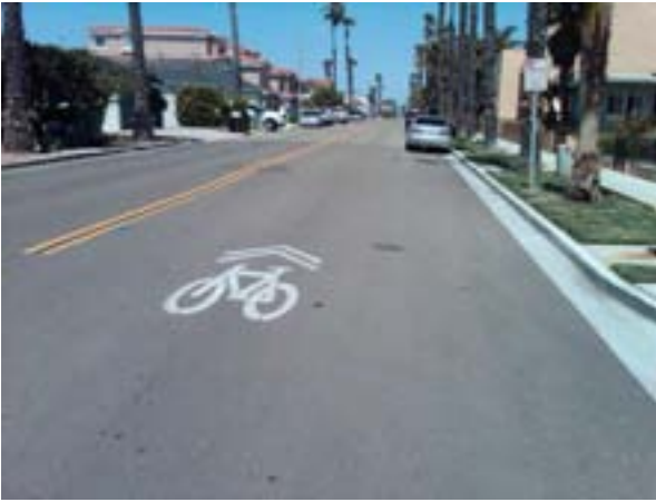
4B) Shared lane markings or “sharrows” remind motorists bicycles can be expected in the roadway and to help cyclists place themselves within the roadway. Photo credit: Joe Punsalan
