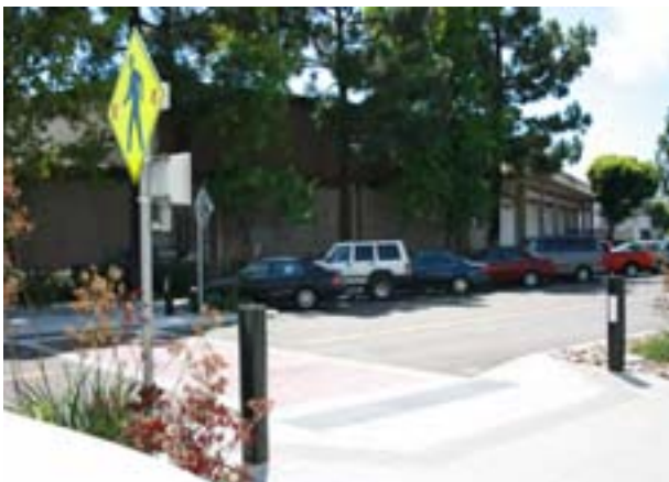
12S) This crossing utilizes lighting in the pavement and in the signs to indicate a pedestrian is in the walkway. Sensors pick up when a pedestrian approaches and if the crosswalk is clear of pedestrians. Photo credit: Joe Punsalan
