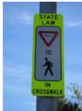
14S) This type of crossing should only be used on streets with one lane each direction or two one way lanes. The center marker is collapsible. It works to slow traffic and concentrate attention on the crosswalk. Photo credit: Joe Punsalan
