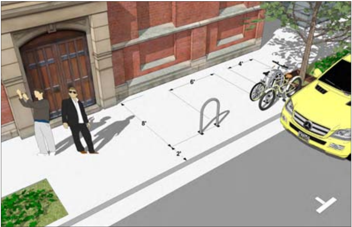
Bicycle Rack dimensions for installation parallel to a curb. Graphic credit: KTU+A
