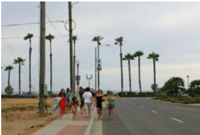
1W) Match the sidewalk width to the intended use. Only suburban residential areas should be allowed at or below a 5' width. Photo credit: Mike Singleton
