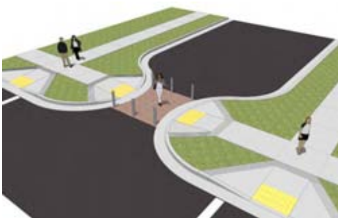
2S) Pedestrian pop-outs in conjunction with bollards can serve to block a street from vehicular traffic. Illustration credit: Michael Johnston
