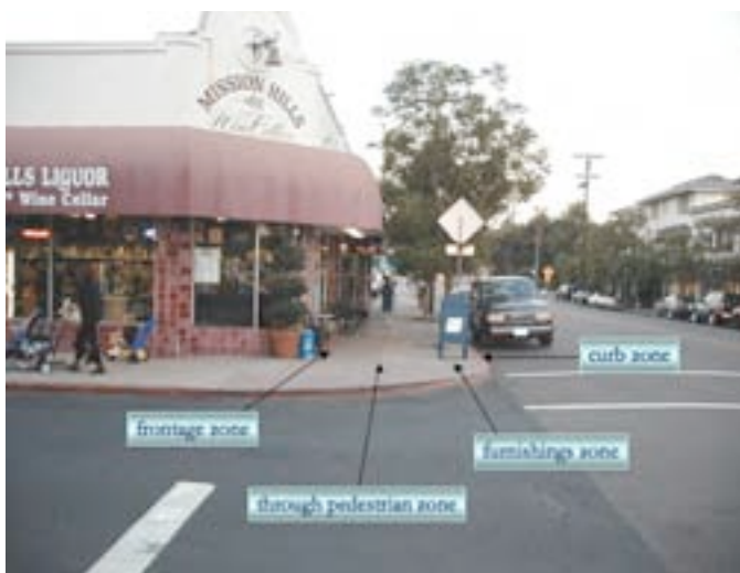
1W) Commercial area widths should approach at least 10' in width since they must accommodate a variety of uses, street furniture and utilities. Photo credit: Andy Hamilton
