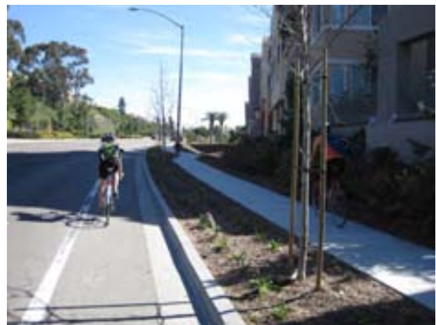
15S) Having an outside striped shoulder or bike lane along with a parkway strip and street trees can dramatically reduce collision potential and increase comfort levels for pedestrians. Photo credit: Joe Punsalan
