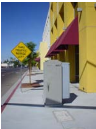
4A) Even though this project provided a wide walkway to start with, some equipment has been placed outside of the furnishings zone and in the throughway zone. Photo credit: Andy Hamilton
