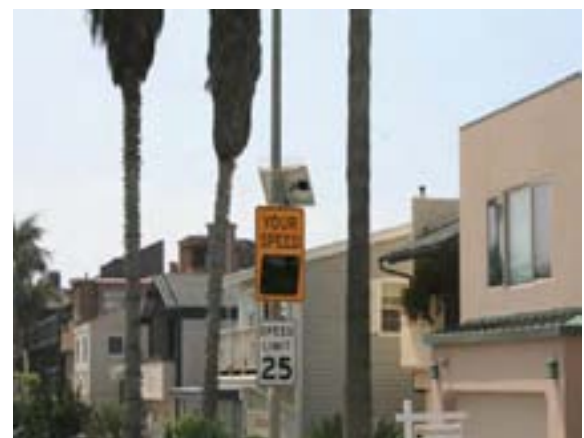
6S) Many cite increased regulation and enforcement as the solution to controlling speeding and reckless driving. Physical improvements provide a long term solution. However, some devices such as radar speed display systems, can help to educate the public and will slow the driver down while in use. Photo credit: Joe Punsalan
