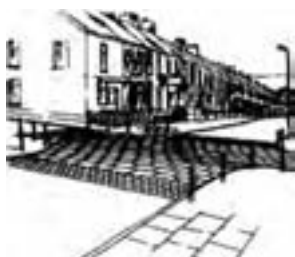
18S) Speed tables (raised intersection). Illustration credit: Dan Burden
