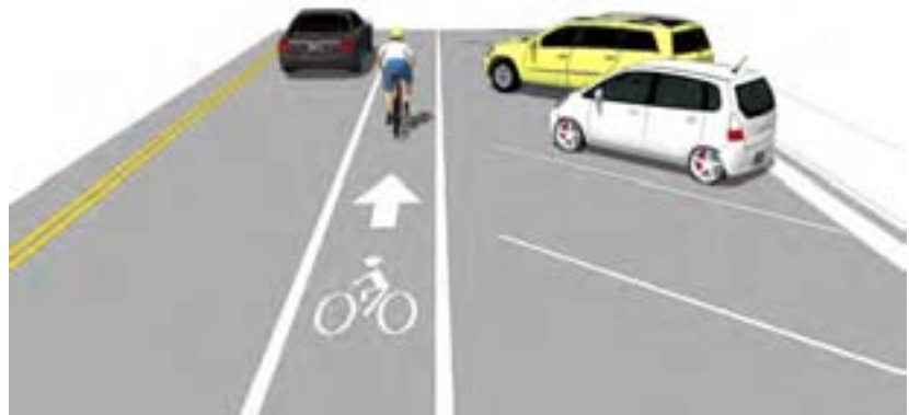
10B) Reversed angled parking allows greater visibility when motorists are exiting a parking stall. Photo credit: Michael Johnston
