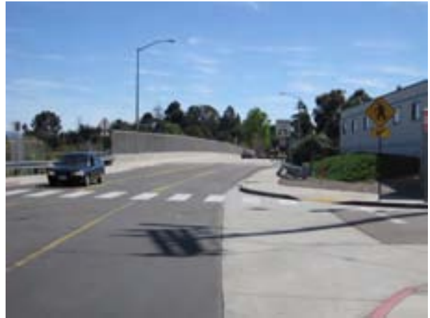
14S) If traffic control is not provided at an intersection, signage and striping along with a center pedestrian zone marker may help to make these crossings as safe as possible. This type of sign may require changes to existing policies, though it is allowed under MUTCD. Photo credit: Joe Punsalan
