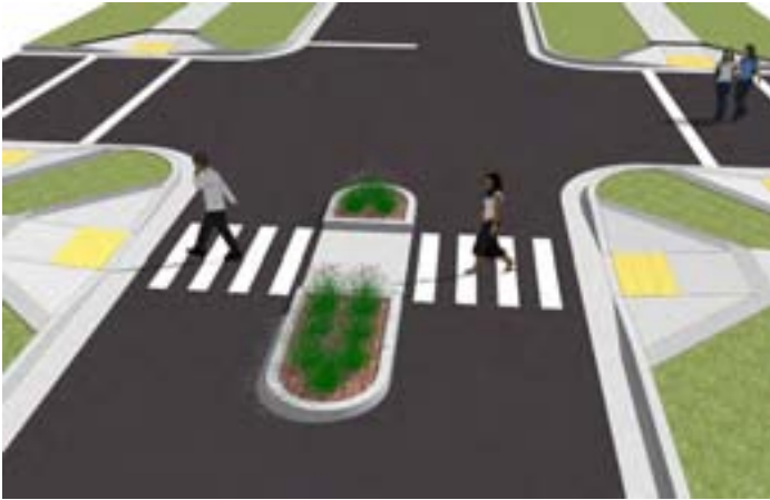
1S) Median refuges should be considered at intersections with or without traffic control. Multi-lane roadways should utilize solutions that include traffic control. Illustration credit: Michael Johnston
