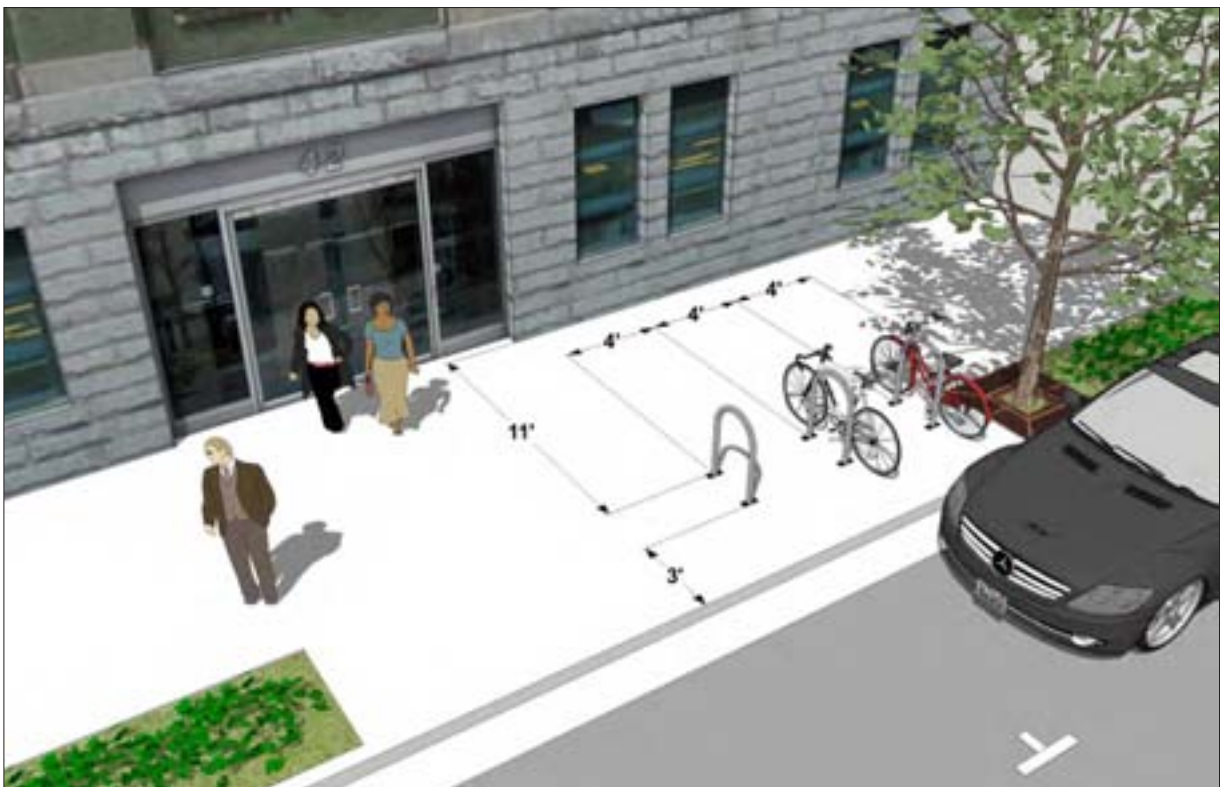
Bicycle Rack dimensions for installation perpendicular to a curb. Graphic credit: KTU+A
