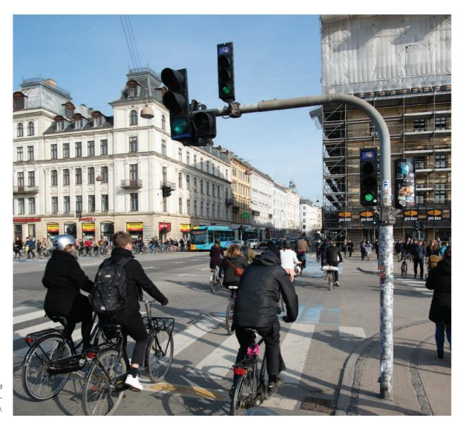
Dedicated bicycle signals can provide a leading bicycle interval, making cyclists especially visible in the intersection.
