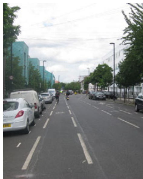
Centre line removed to allow advisory cycle lanes to be introduced past parking, London
