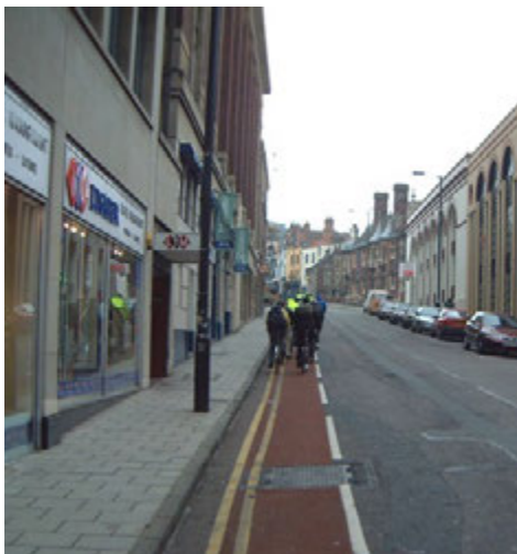
Advisory cycle lane in uphill direction only, Bristol. Note that the cycle lane width is less than the 1.5m recommended minimum and does not enable cycle users to overtake within the lane.
