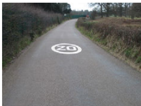
20mph roundel and omission of centreline on a rural lane, Devon
