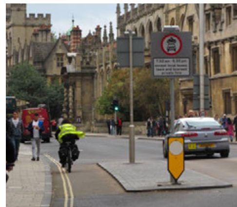
Bus gate with separate cycle bypass at entry to time-limited vehicle restricted area, central Oxford. Cyclists share the carriageway with buses and taxis
