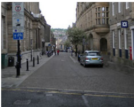
Cycle access to time-limited pedestrian zone, with unsegregated contraflow cycling, Church Street, Lancaster
