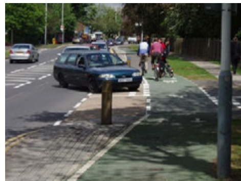
Cycle-only track crossing of low flow access road with priority over side road. The set back is less than 5m, which helps retain the cycling desire line. Hillingdon, West London
