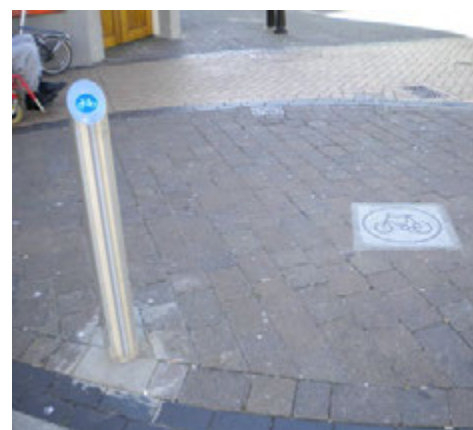
Cycle route diagram 955 on a bollard and an adaptation of diagram 955 as a paviour in a pedestrianised street near Blackpool Tower
