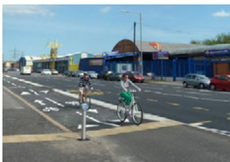
Segregated shared use cycle track with raised platform at bus stop and transition to unsegregated shared use at controlled crossing of the adjacent road, Belfast
