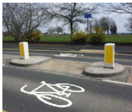
Cycle symbol (Diagram 1057) in centre of traffic lane at carriageway narrowing, London
