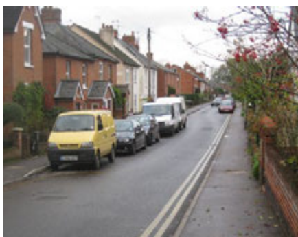
Residential street traffic calmed by removal of centre line and positioning parking on alternating sides of carriageway, Wokingham
