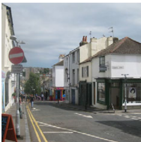
No entry except cycles provides cycle access to unsegregated contraflow cycling, Brighton
