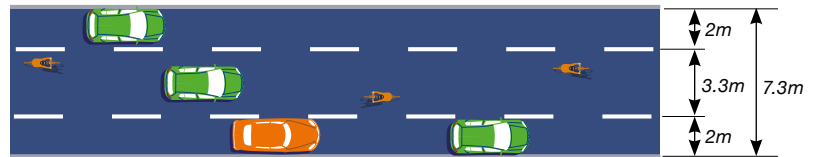
Figure 3.5 Typical layouts with contraflow cycling
