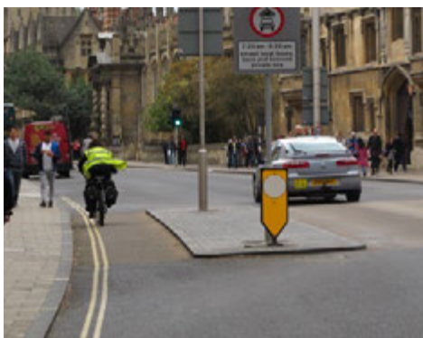
Time limited vehicle restricted area controlled by signed bus gate, central Oxford. Cyclists share the carriageway with buses and taxis
