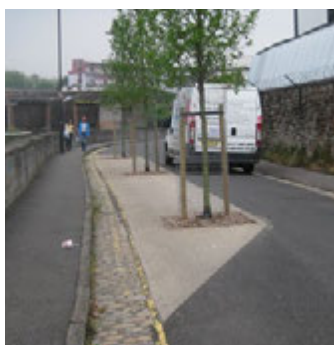
Removal of centreline and trees planted in the carriageway create informal traffic calming on a radial cycle route into central Bristol
