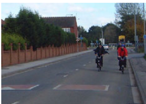
Cycles share mixed traffic lanes calmed with Speed cushions, Nottingham
