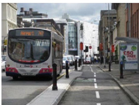
Cycle track raised to footway level and locally narrowed to create a bus boarding area and to moderate cycling speeds, Glasgow
