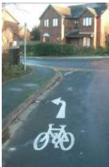
Diagram 1057 with direction arrow (diagram 1059)
