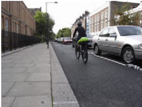
Light segregated cycle lane using Armadillos, Camden London
