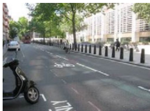
Diagram 1057 indicating cycle riding position where traffic lane is narrowed by parking, London
