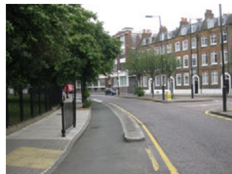
Cycle track with kerb segregation, Islington, London. The margin strip is splayed to minimise the risk of cyclists colliding with the outer edge of the narrow track
