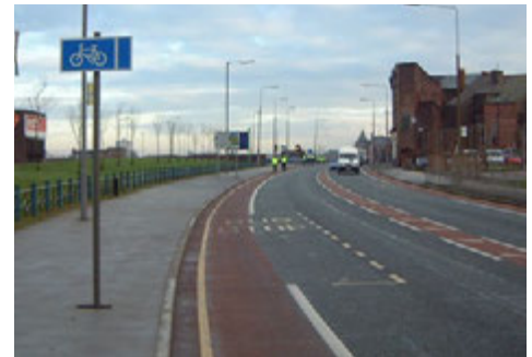
Mandatory cycle lane discontinued at bus stop cage, Liverpool. Coloured surfacing provides visual continuity when a bus is not at the stop
