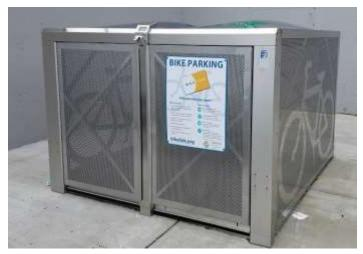
Figure 4.11. Bike lockers are an example of long-term, secure bicycle storage.
