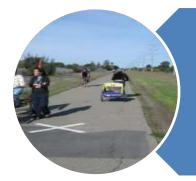
Shared Use Paths (Class I) are two-way paved facilities, physically separated from motor vehicle traffic and used by bicyclists, pedestrians, and other non-motorized users. Shared use paths are often located in an independent alignment, such as a greenbelt, flood control channel park, or abandoned railroad.
