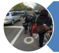
Bike Lanes (Class II) provide an exclusive space for bicyclists in the roadway. Bicycle lanes have established painted lines and symbols on the roadway surface. Bicycle lanes are for one-way travel and are typically provided in both directions on two-way streets and/or on one side of a one-way street.
