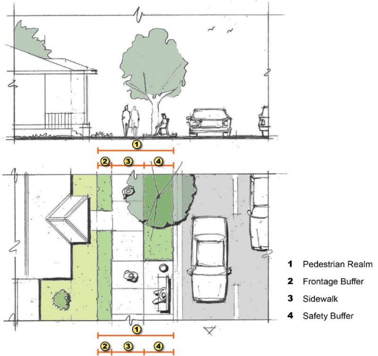
Figure 17.4 – Pedestrian Realm Components
