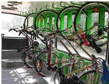
Figure 19: Segregated device for hanging Bicycle (Brno)
