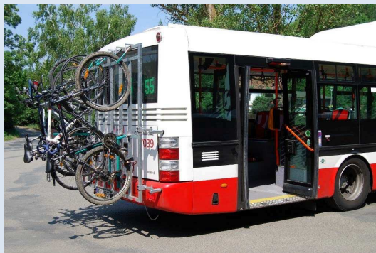
Figure 12: Brno newly introduced Backside rack within CIVITAS Plus II 2MOVE2
