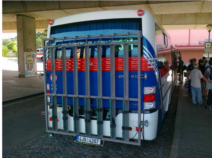
Figure 8: Backside rack in regional bus in South Moravian Region (Czech Republic)
