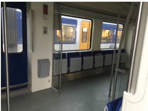
Figure 24: Fixed device for bicycle, flexible chairs (the Netherlands)
