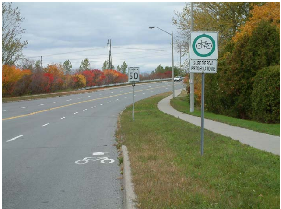
Exhibit 5.9 Wide Curb Lane with Bicycle Pavement Markings and Signing (City of Ottawa)
